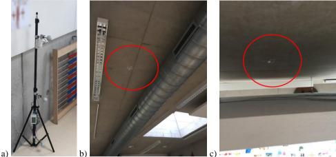
**Fig. 4.** a) The measurement stand used in the classrooms, b) Surface temperature measurement on the ceiling surface facing the room, c) Surface temperature measurement on the ceiling surface covered by the acoustic sound absorber.
