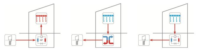
Fig. 1 (1) Heating mode, (2) passive cooling mode, and (3) active cooling mode [2]
